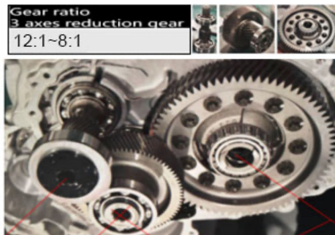
Figure 7: 12:1~8:1 ratio gear reduction [1]
